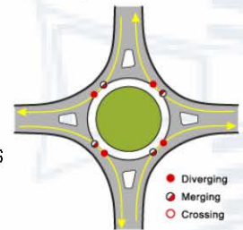
A comparison of conflict points: A four-way intersection vs. a modern roundabout
