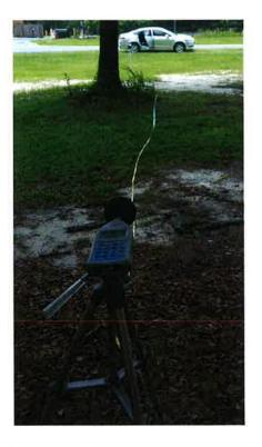
Figure A.2: SC – Ambient Noise Monitoring Setup 1, Receptor 1.2
