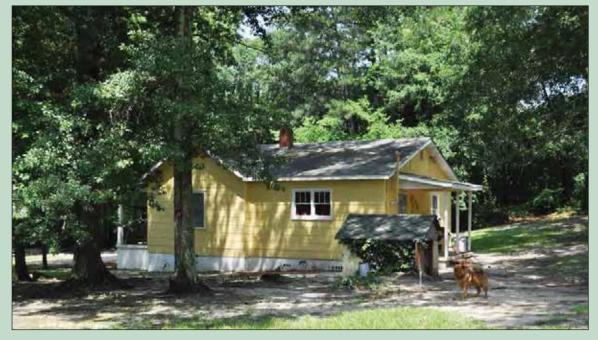
Just east of the house is a rectangular well house with a front-facing gabled roof. Constructed of concrete block, the small building includes gables clad in metal sheeting. A single plywood door is situated in the northeast elevation and its gabled roof is covered in asphalt shingles.
