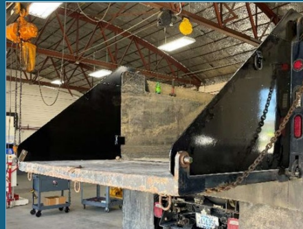
Donald Mahoney—Debris Chute (Clarendon Maintenance, D7)
