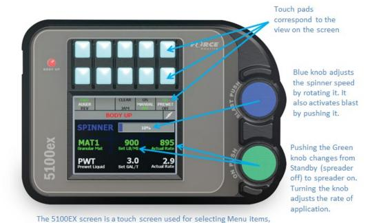
The 5100ex Controller will automatically power up when the truck is started, but <u>only</u> press Continue if you plan to use the system.
