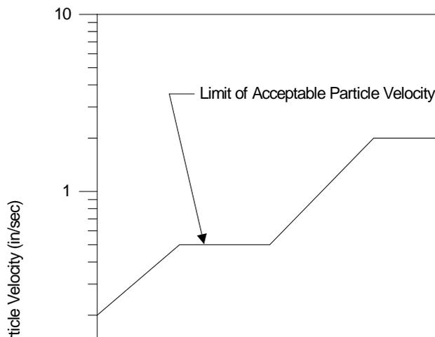
Figure 1 - Vibration Criteria (adapted from AASHTO R8-96)
