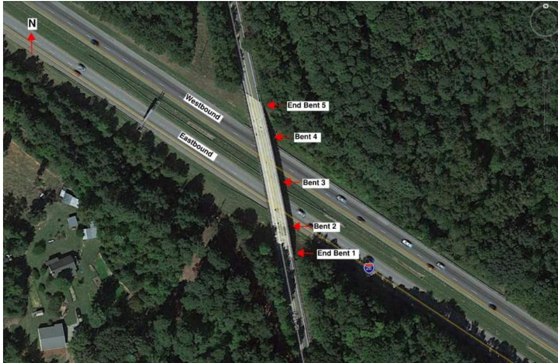
Figure 3 - Existing Bridge Layout
