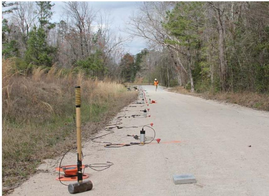
**Figure 15** *Looking north at 4.5 and 1 Hz geophones along Conway MASW Arrays 1 and 3*
