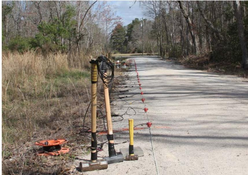
**Figure 16** 1.5 kg hammer, and 4.5, and 9 kg sledgehammer energy sources at south end of Conway MASW Array 2
