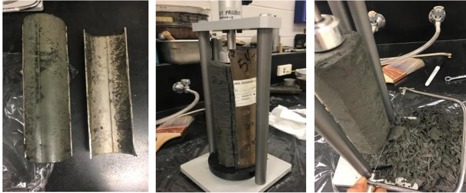
**Fig. 1** Soil Sample Preparation: (a) Cutting, (b) Removing Tube and (c) Trimming
