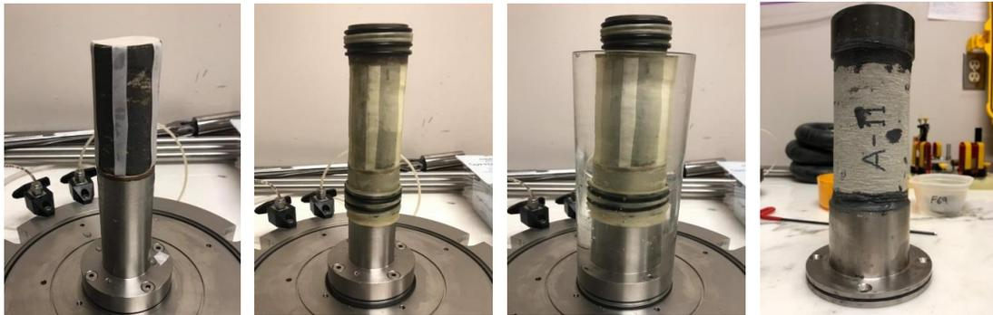
**Fig. 3** Sample Setup in RCTS Device: (a) Disc Filter Paper and Filter Drainages, (b) Radius Drainages Installation with Soil Sample, (c) Rock Sample Installation on Bottom Plate and (d) Top Cap Installation above Rock Sample
