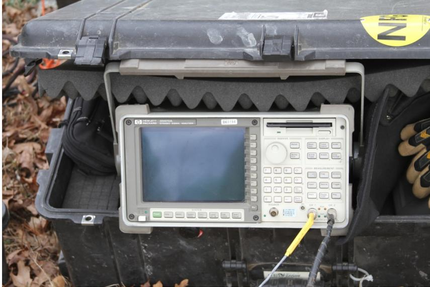
*Figure 18 HP 35670A dynamic signal analyzer used for SASW acquisition*
