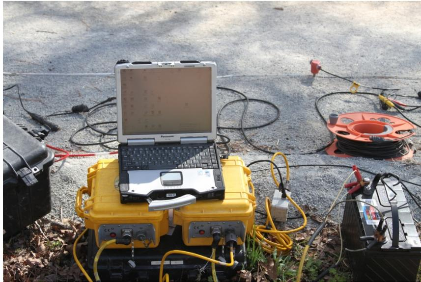
**Figure 14** *Geometrics Geode seismograph*
