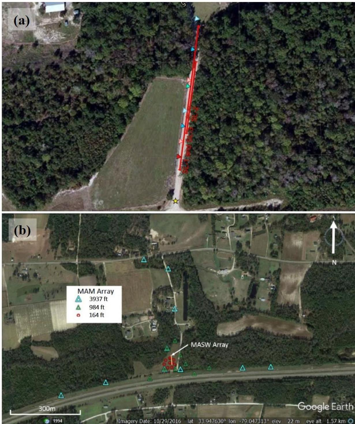
**Figure 3.3** Surface Geophysical Testing Locations at Site A: (a) MASW and SASW Testing Arrays, (b) MASW and MAM Testing Arrays
