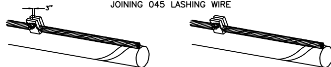
TYPICAL DETAIL – G JOINING 045 LASHING WIRE
