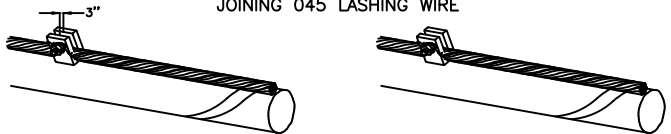
TYPICAL DETAIL – G JOINING 045 LASHING WIRE
