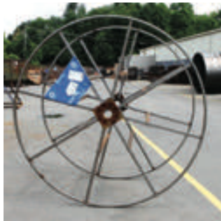
8-10 spoke Construction Clip or Bolt-in place Stave
