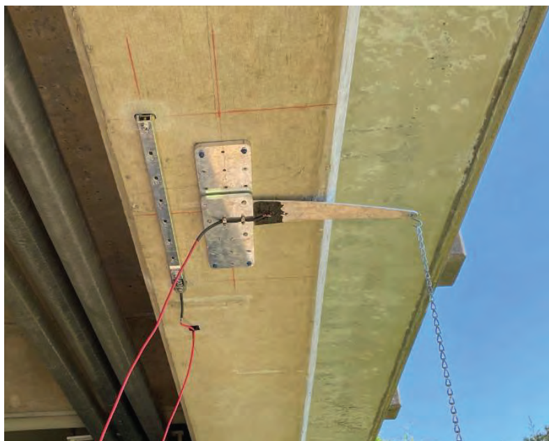
Figure 8: Installed Instrumentation BR 2827
