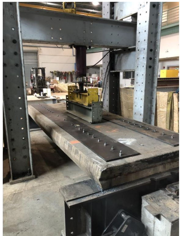
Figure 3.5 Strengthened slab test setup with two plates on top.
