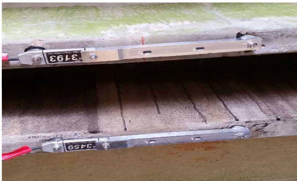
Figure 8: ST350 Strain Transducer with 9-in. extension arm.
