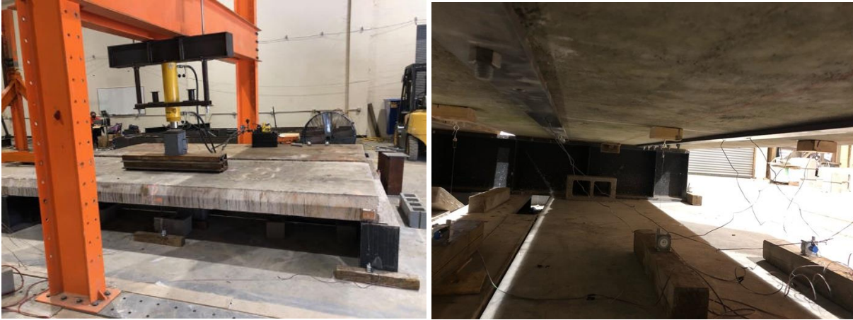
Figure 3.13 Strengthened slab test setup and ready for loading (left). Two plates installed on bottom of slab (right).
