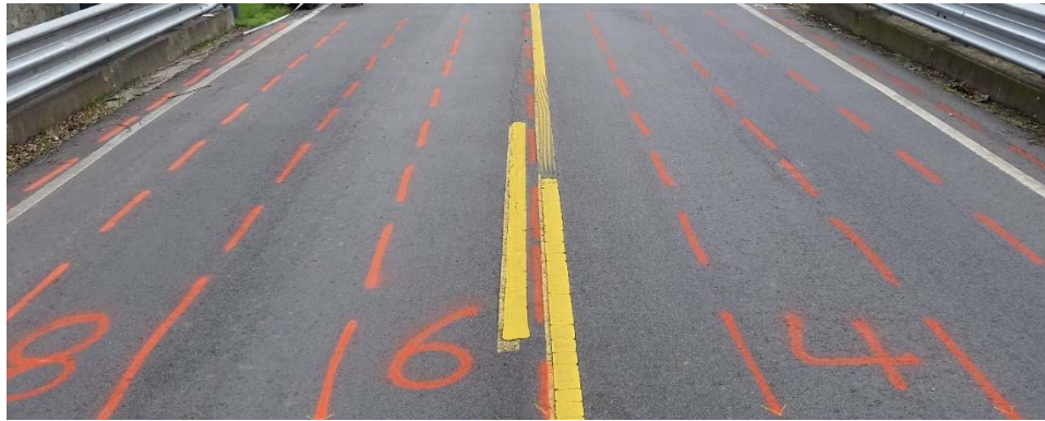
Figure 19 Temporary Marking Lines on the Bridge Deck for Proper Truck Alignment During the Load Test
