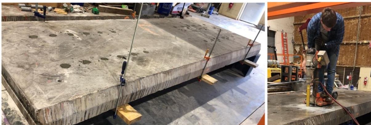
Figure 3.12 Installation of bolts and grout of the strengthened slab with steel plates from bottom. Wood planks, clamps, and grout are shown in the left photo; hole cutting is shown in the right photo.
