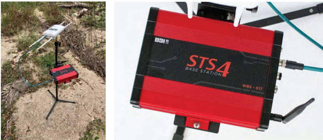
Figure 6: STS4 System used in the Load Test (BDI)
