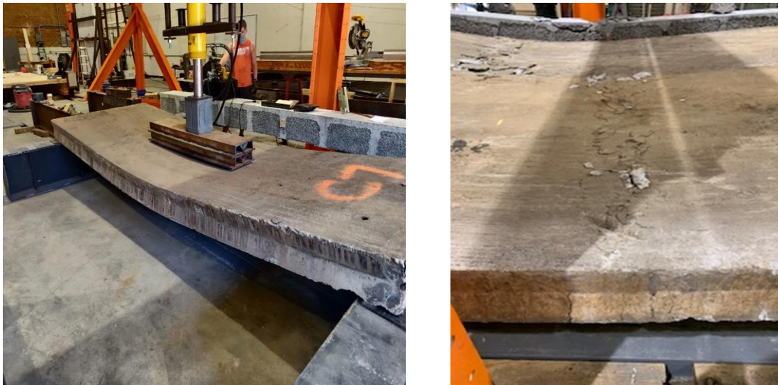
Figure 4.3 Deformation (left) and concrete crushing (right) of the flat slabs.
