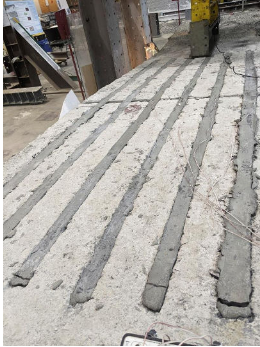
Figure 4.10 Debonding and cracking of grout
