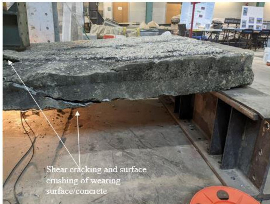
Figure 4.9 Failure mode of NSM test
