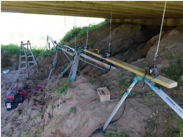
Figure 17: Wide-leg Channel Bridge Installed with Cable Potentiometer (Typ.)
