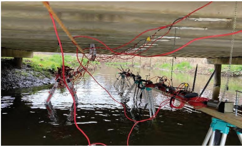
Figure 15: Wide-leg Channel Bridge Installed with Strain Gauge (Typ.)
