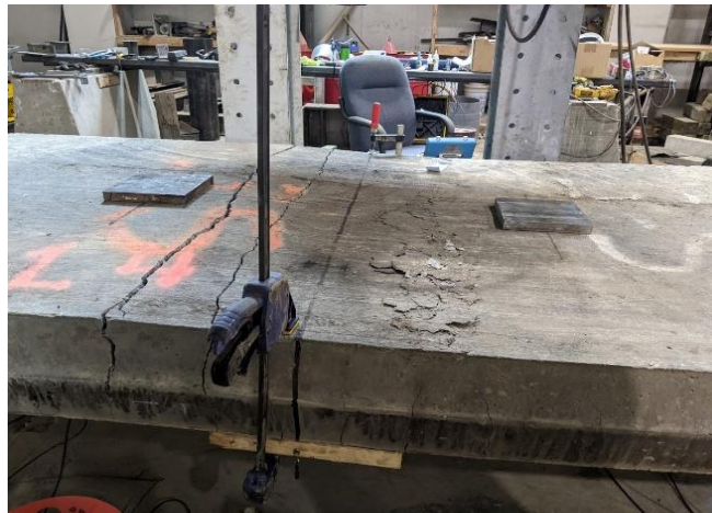
Figure 3.24 Damage slab specimen
