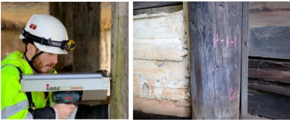
Figure 7.1 In field use of a resistance drill (left photo) and the field marking of a timber pile that has been drilled (right photo).
