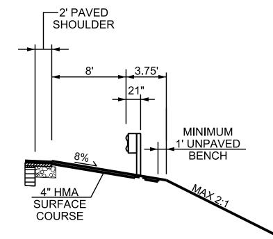
STANDARD GUARDRAIL DETAIL WITH ASPHALT NON-MOW STRIP
