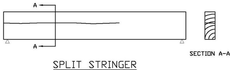
Figure 13.2-1. Cracked, Broken and Split Timber Stringer Defects
