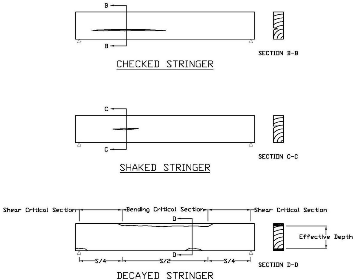
Figure 13.2-2. Checked, Shaked and Decayed Timber Stringer Defects
