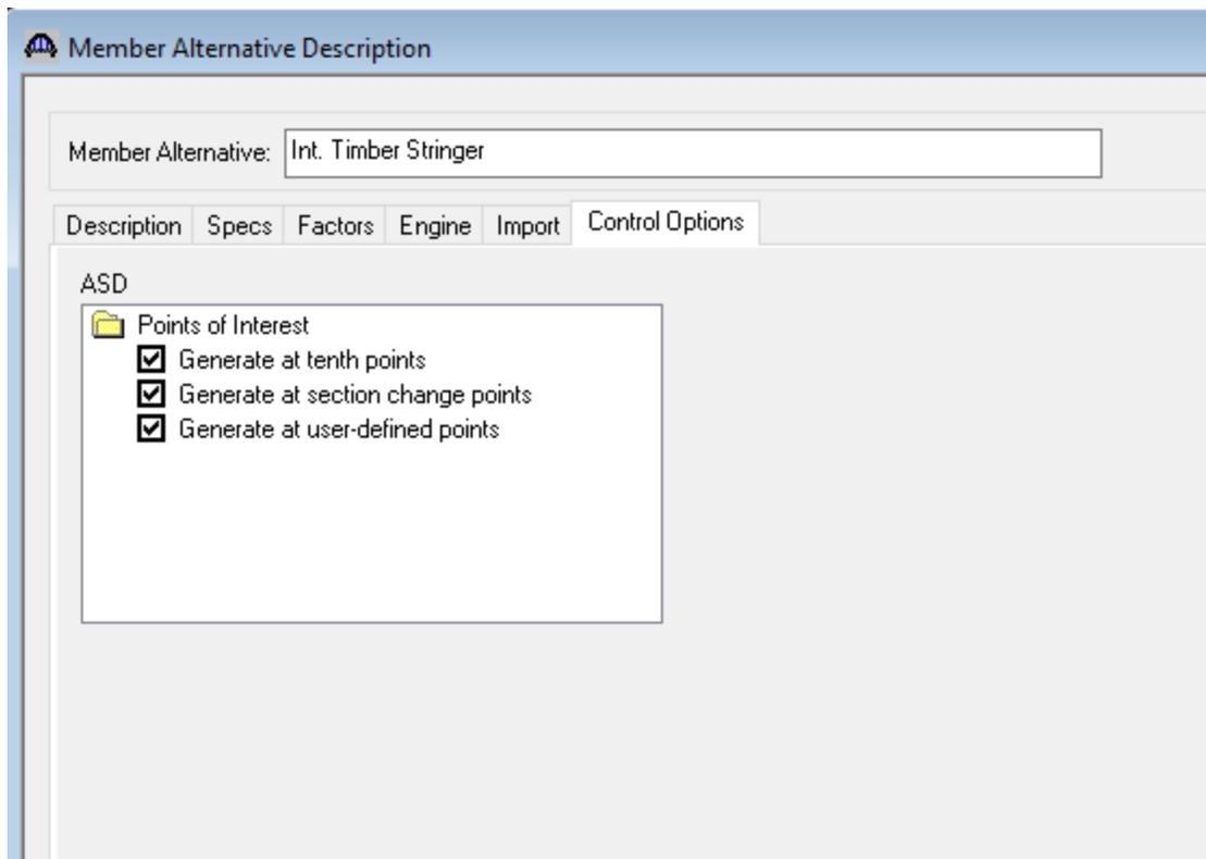
Figure 13.2.1.1-1. Control Options in BrR for Timber Superstructure
