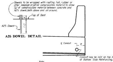
Conduits necessary for utilities to be furnished by the utility company and placed at no expense the department. Use Slip Coupling on Conduits at Expansion Joints.
