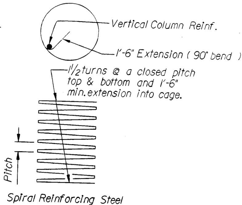
This detail should be used at both ends of each spiral column reinforcing cage, unless required otherwise by design. Designs and plans previously completed need not be revised to comply with this memorandum.
