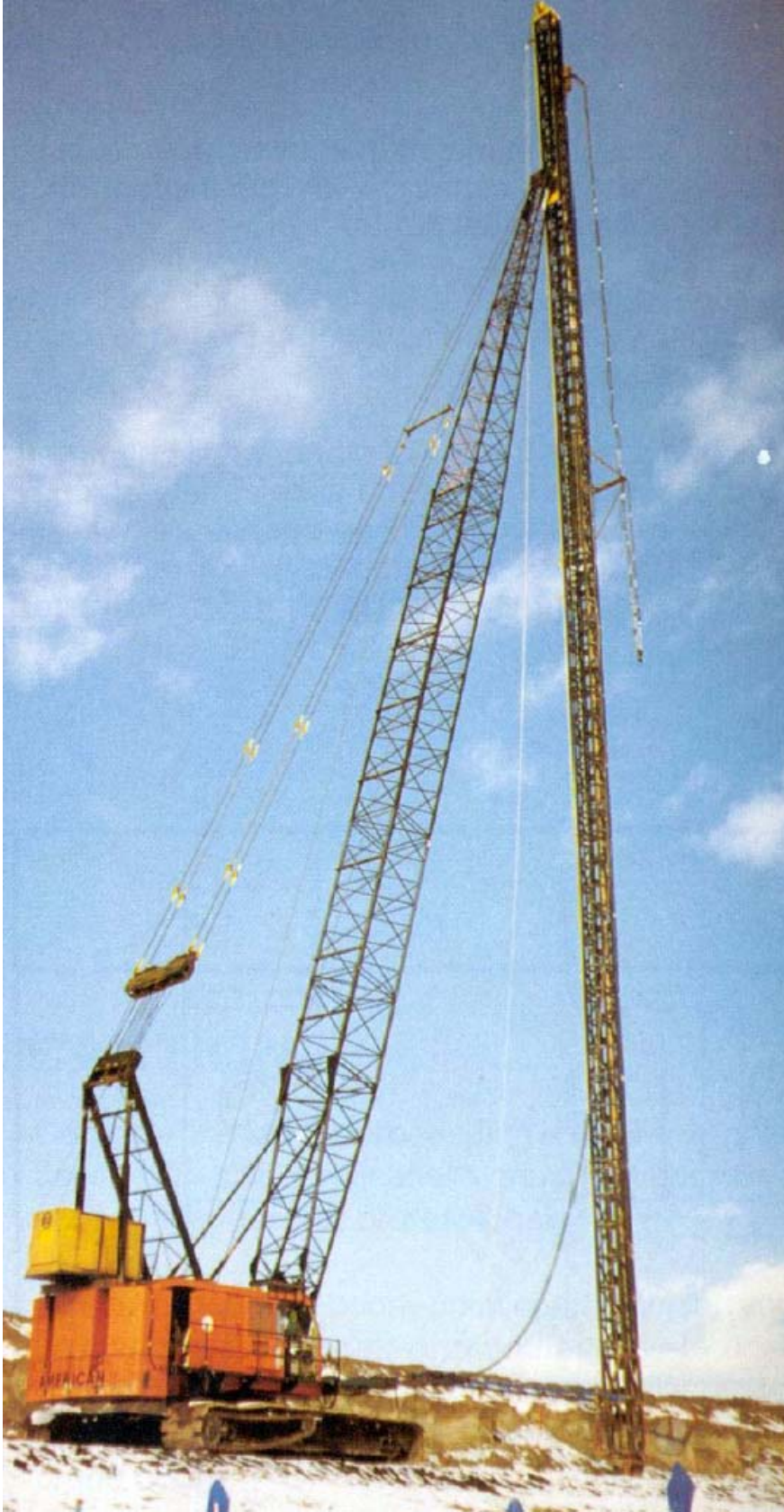
Photograph of Crane-Mounted Wick Drain Rig.
