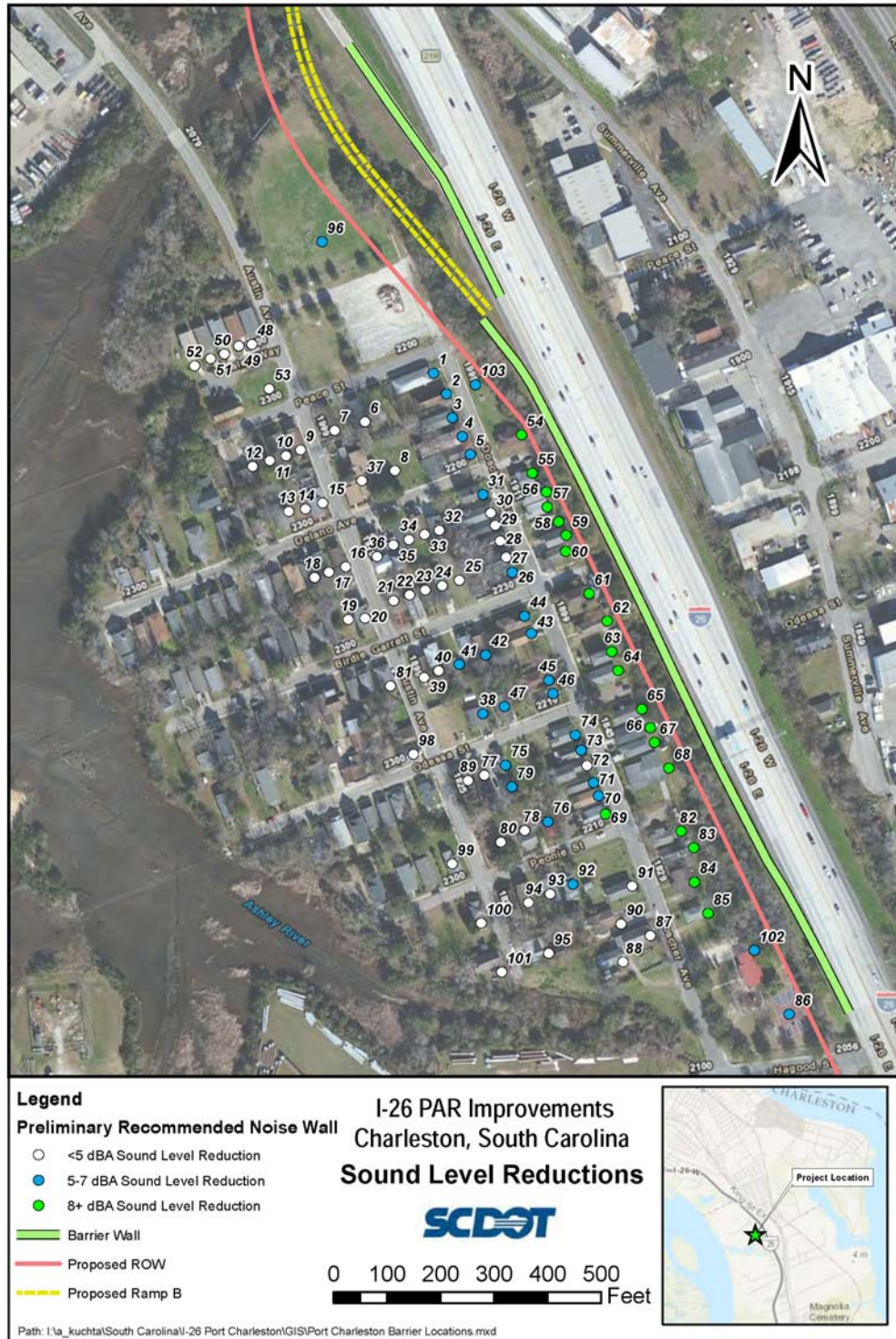
Figure 3 – Preferred Noise Barrier Placement and Results
