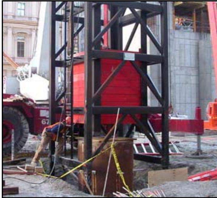
**Figure 24-5, High-Strain Load Testing Apparatus
