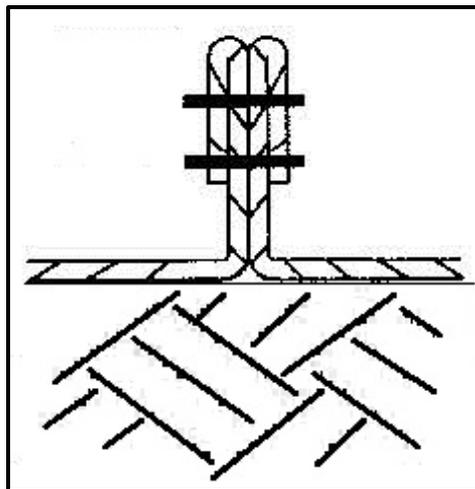
**Figure 20-4, Proper Seam Placement
