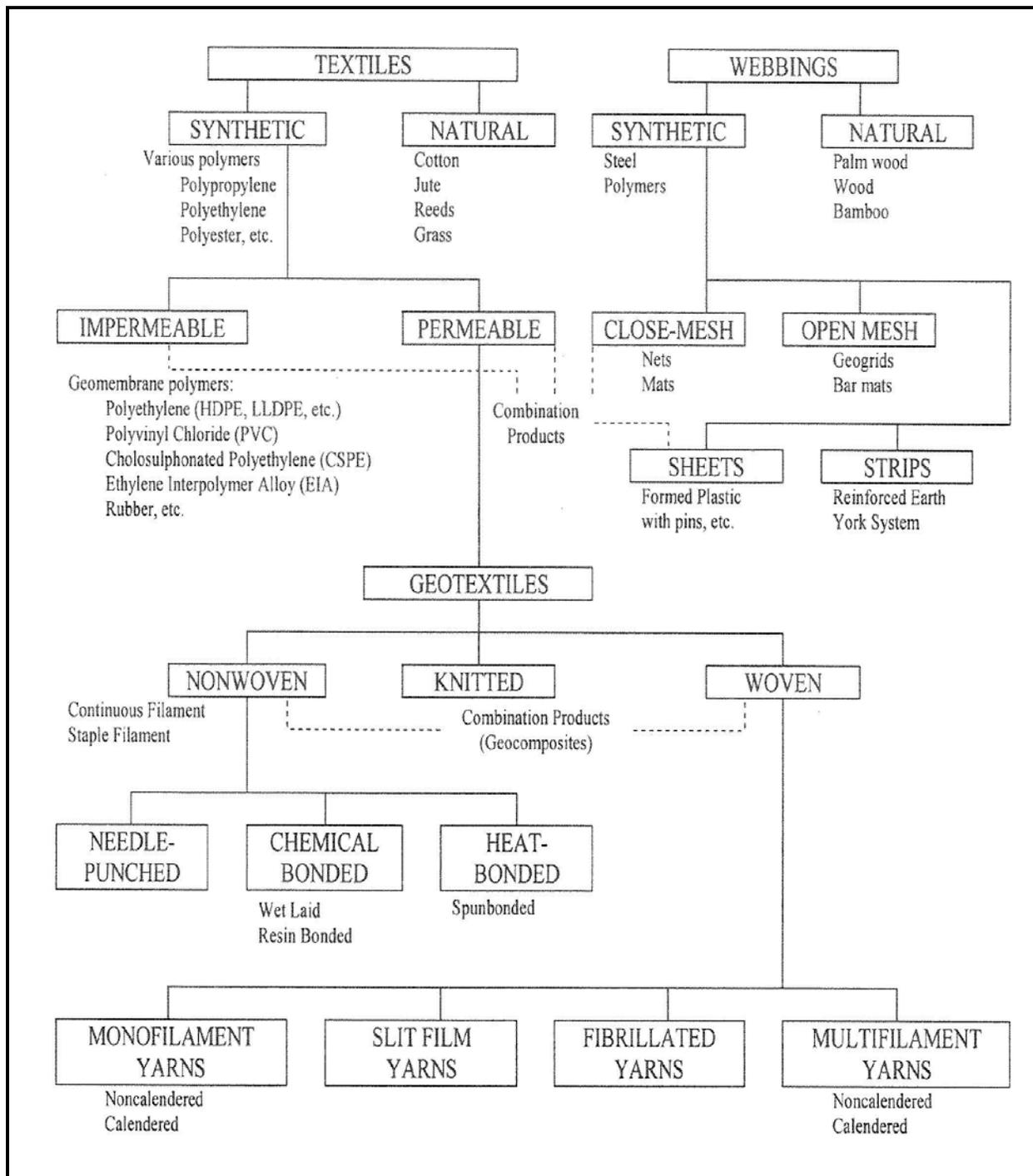
**Figure 20-1, Geosynthetic Classification Scheme (Holtz, et al. (2008))**
