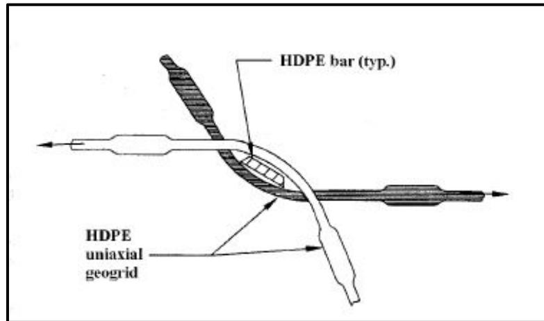
**Figure 20-6, Geogrid Mechanical Connection
