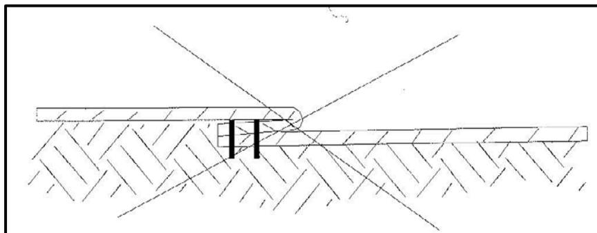
**Figure 20-5, Improper Seam Placement
