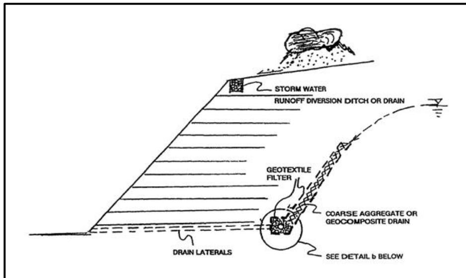
**Figure D-14, Groundwater and Surface Drainage
