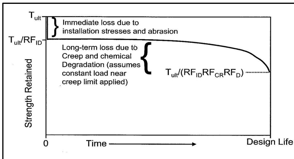
**Figure D-5, Long-Term Geosynthetic Reinforcement Strength Concept
