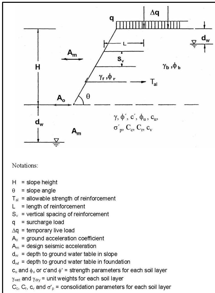
**Figure D-1, RSS Design Requirements and Geometry
