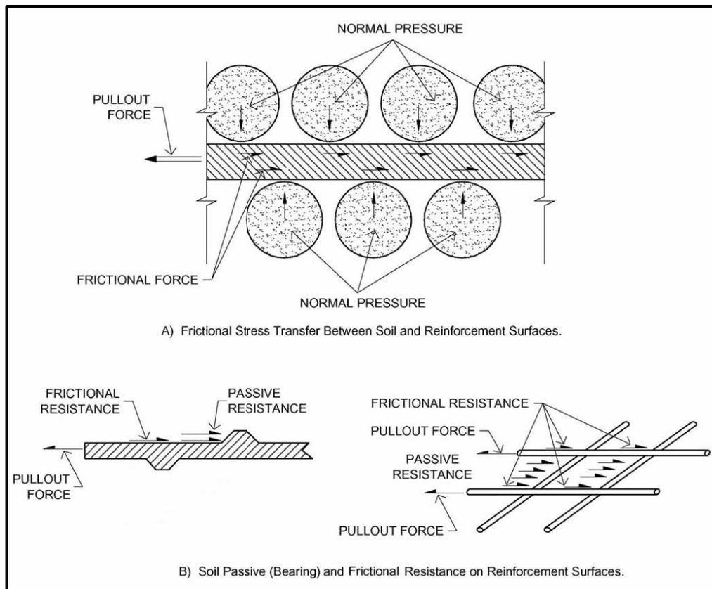
**Figure D-2, Mechanisms of Pullout Resistance
