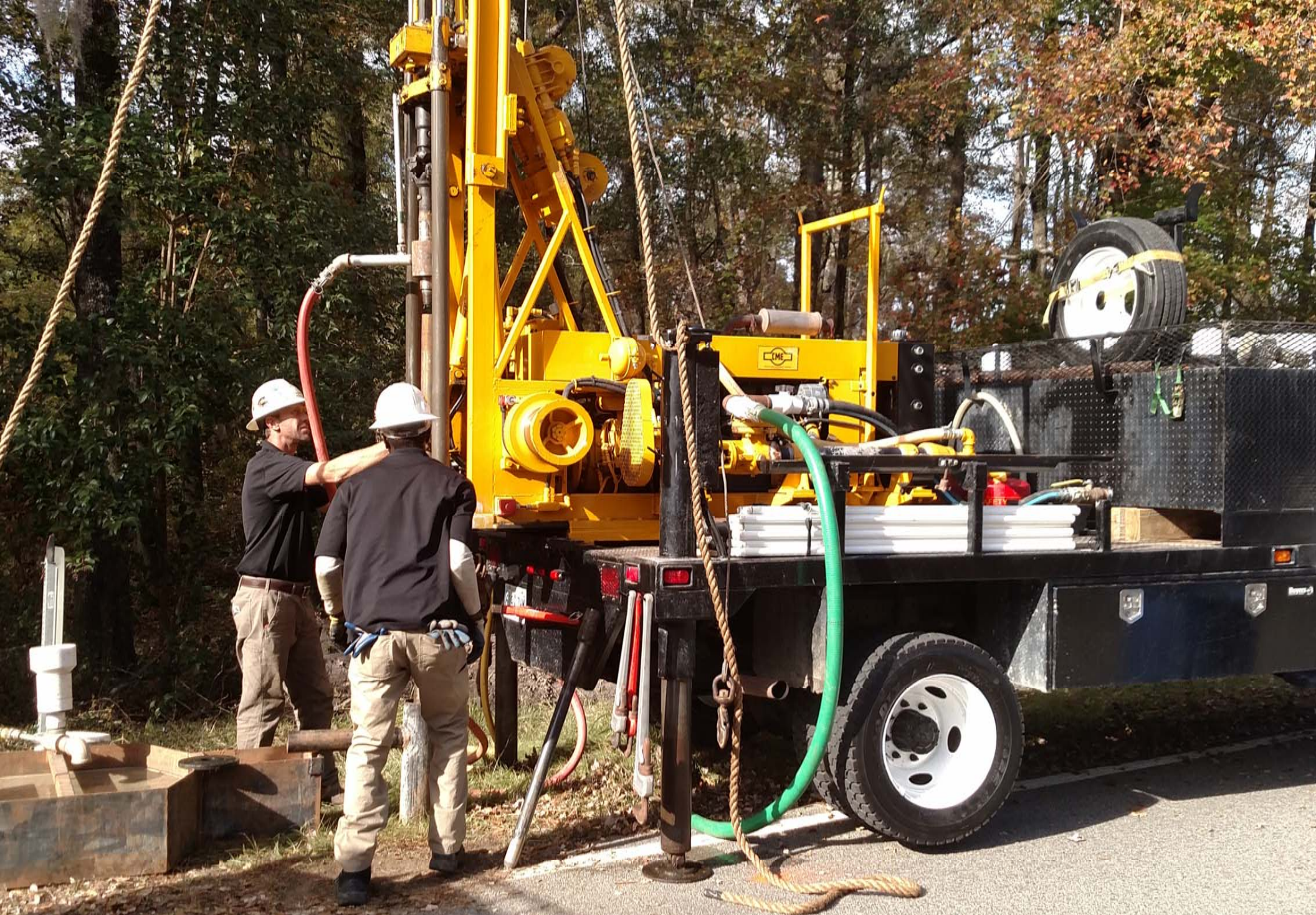
Figure No. 3: Photograph of Soil Test Boring STB-101 Being Drilled
