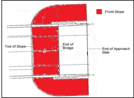
Figure - Front Slope Definition
