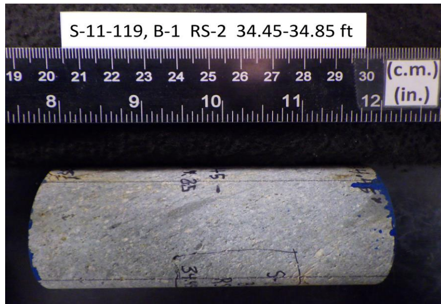
After cutting and grinding
