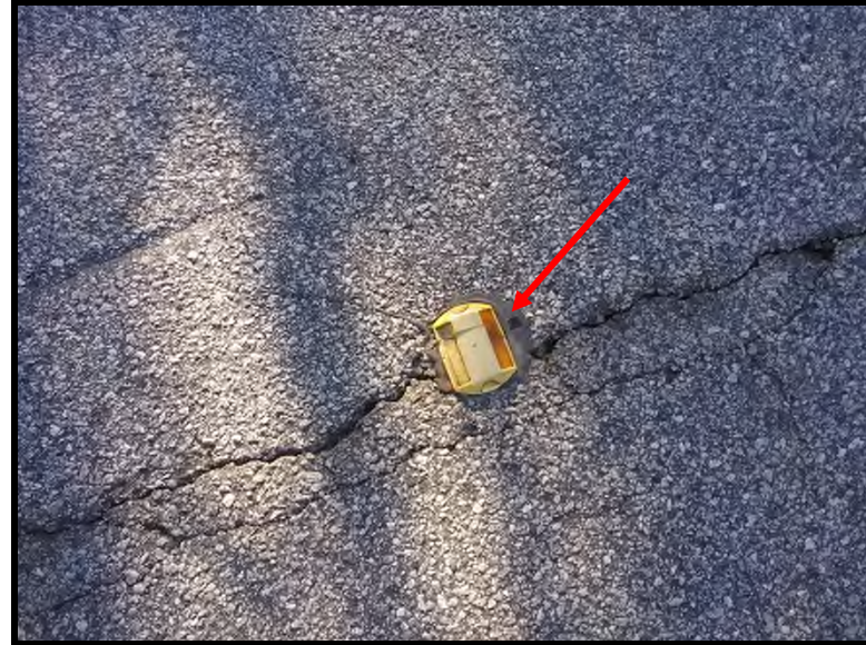
2 Puck mastic associated with the reflectors tested negative for asbestos.
