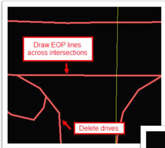
**Edit** the existing edge of pavement graphics further to connect lines and arcs for the edge of pavement. **Remove** drives and **join** lines through intersections. Close the shapes at the beginning and end of the project.
