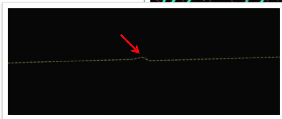
The following example shows a dip in the elevation along the left edge of pavement of the travel lane.
