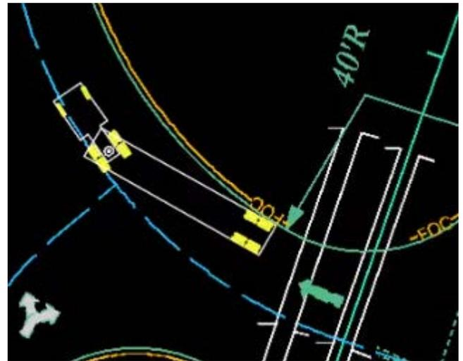
**Modify** the intersection design radius if necessary. **Modify** the truck turning path if necessary to ensure good movement.
