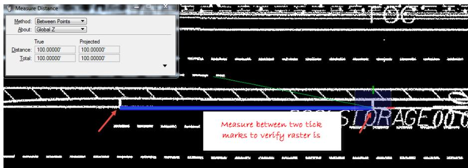
To **clip a map**, draw a fence with the approximate center location. Select the **Clip** tool, toggle Method: **Fence** and Mode: **Clip Boundary**. Data clip to accept the clip.
