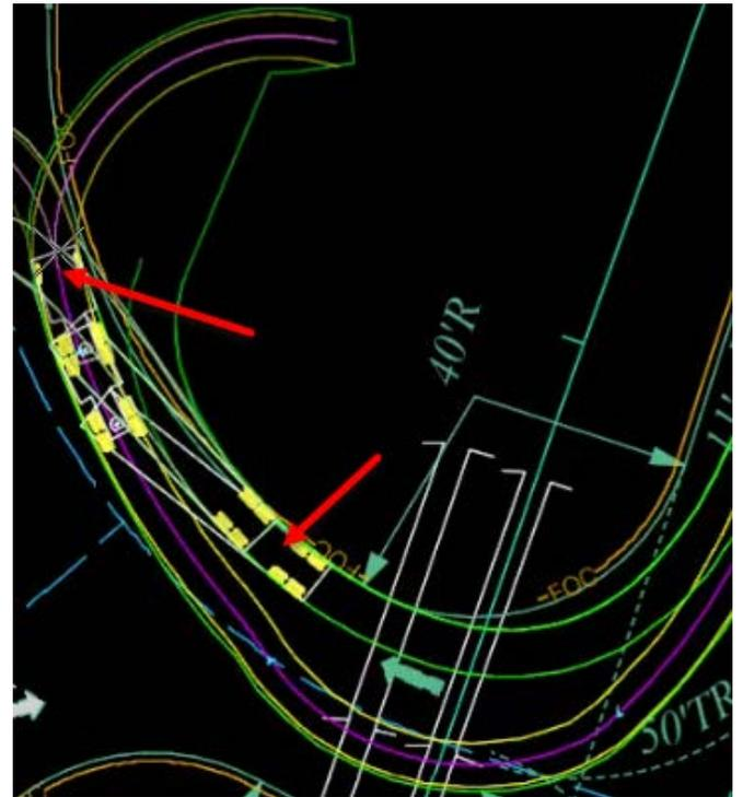
After completing the path, press the **Path Control** icon. This will highlight the path with Nodes that can be moved (right image below). Use the mouse to drag/drop and fine tune the vehicle path to fit onto the road and turn radius of the intersection (bottom image).
