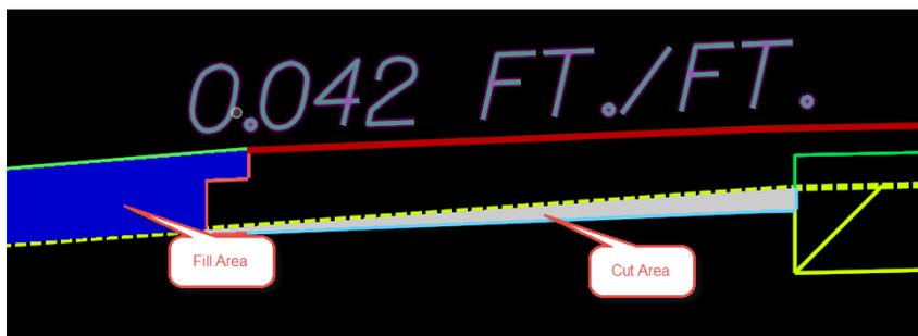
**Turn OFF** the **RD\_XS\_EwShp level** and select **File > Save Settings** (or Ctrl + F). This keeps the shapes from plotting on the cross section sheets.
