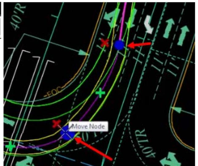
Press the **Run Animation** icon and select the path. The **Hide Simulation** can be checked on or off for viewing the vehicle movements. The **Loop Animation** button can be turned on to repeat the simulation again. Set the timing to 5 seconds and press the **Play** button to review the movements.
