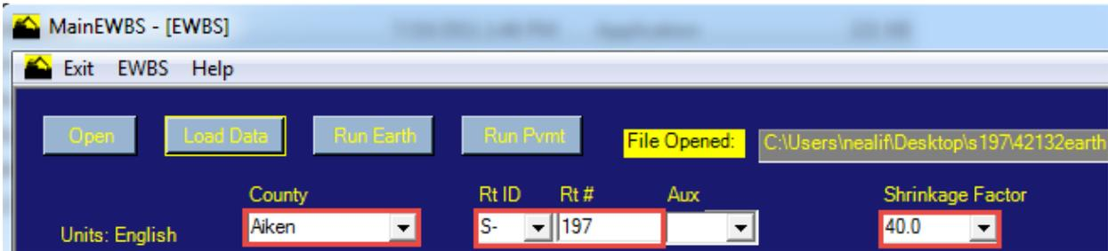
For the **Shrinkage Factor**, refer to the map area for the County to determine whether to use 30% or 40% unless otherwise directed by the Engineer of Record.
