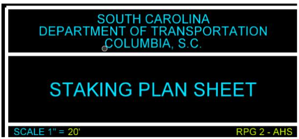
Scale the text to a legible size when plotted, use the same multiple as used for the 05\_Staking\_Plan\_Sheet cell. In this example, you will need a minimum font size of 5. Larger fonts can be utilized to distinguish notes and labels.
