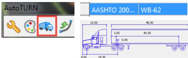
To create a turning path using **Path tools**, select the 4<sup>th</sup> icon, **Generate Arc Path**. **Data click** the vehicle into the lane approaching the intersection. Rotate the vehicle and data click again to place the vehicle in the correct direction.
