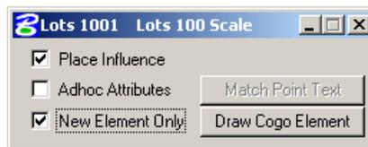
From the secondary dialog that is opened, click the Draw Plan & Profile button to initiate the drawing of COGO elements into the design file. Clicking this button prompts the user for a job number (the coordinate geometry database file wherein the COGO elements are stored), and then opens a dialog that enables the user to choose a COGO item to draw. Do Not activate the Place Influence toggle when using Draw Plan & Profile.
