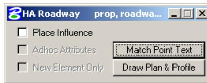
**Adhoc Attributes** is used with **Place Influence** to add Adhoc Attributes to any new element when that element is drawn. A table is displayed when a MicroStation command is selected and the user can modify the value of the Adhoc Attribute prior to placement of the element.
