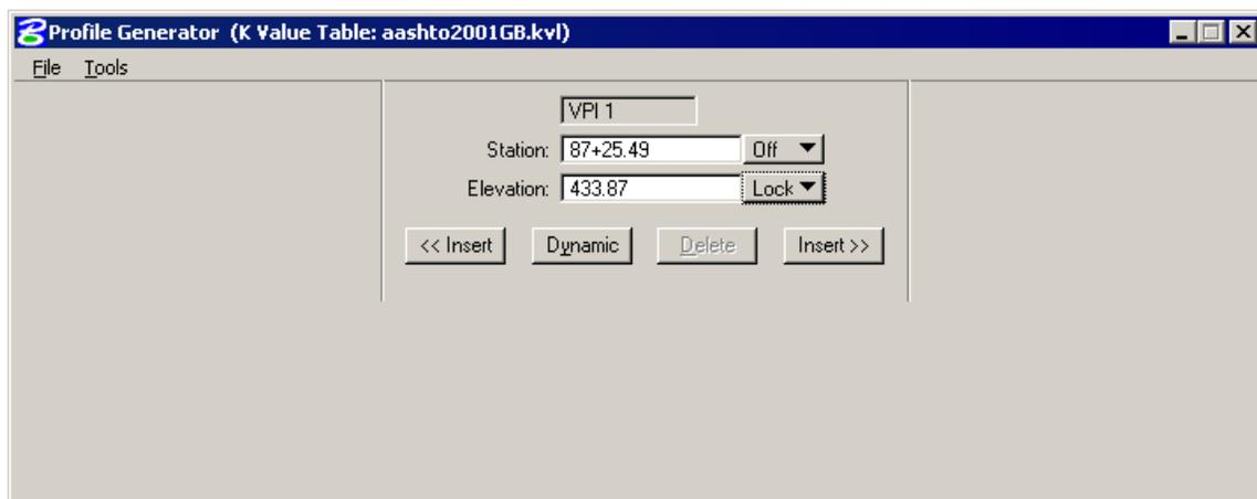
7. Click the **Insert After** button and complete the VPI Station and Elevation of the subsequent VPIs as detailed in the table below.
