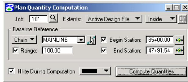
Once the MicroStation plan view design file is accessed, the first step is to invoke the Design and Computation Manager and click the shortcut button at the top of the dialog to Compute.
