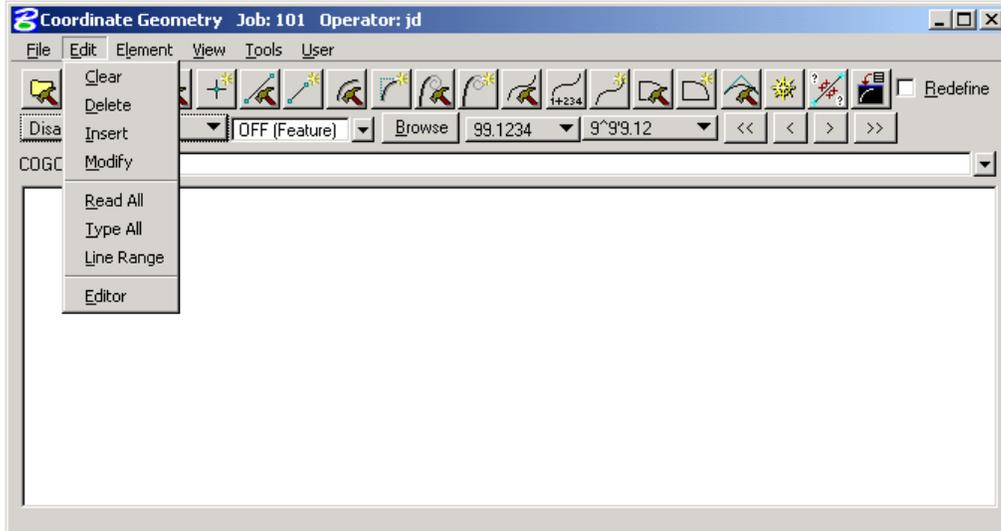
**Clear** Empties the memory of the current audit trail without saving and initializes the line numbers to begin a new sequence of commands. Note this does not clear the display window.
