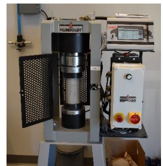
QC Team's AASHTO Accredited Lab Concrete Compression Testing Apparatus
