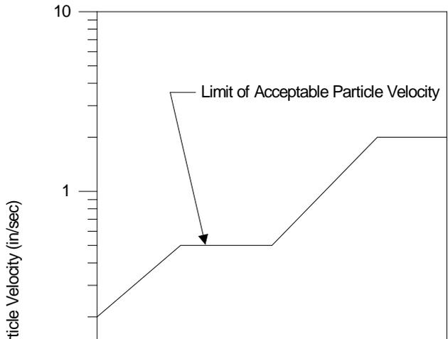
Figure 1 - Vibration Criteria (adapted from AASHTO R8-96)
