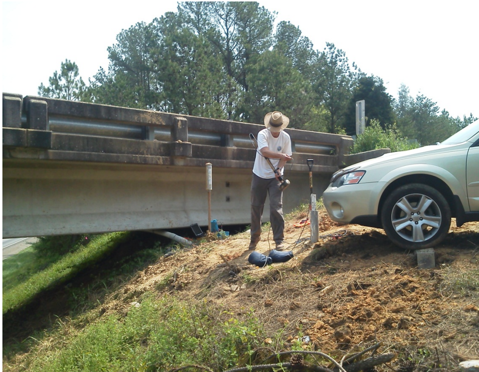
8. Downhole Shear Wave Velocity Testing on boring B-2A.
