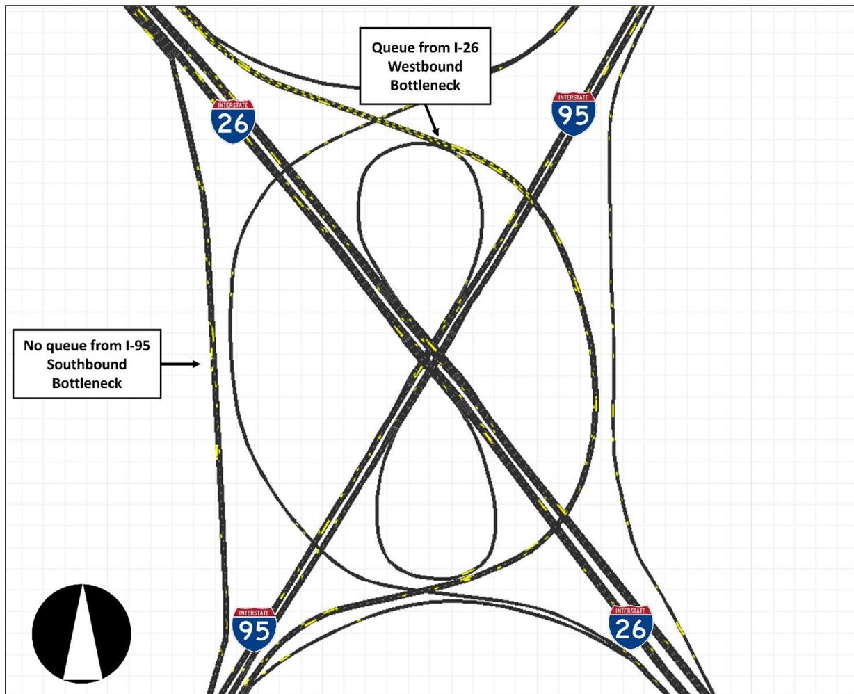
**Figure 7.5: TransModeler Alternative 2 (I-26 Additional Widening)**
