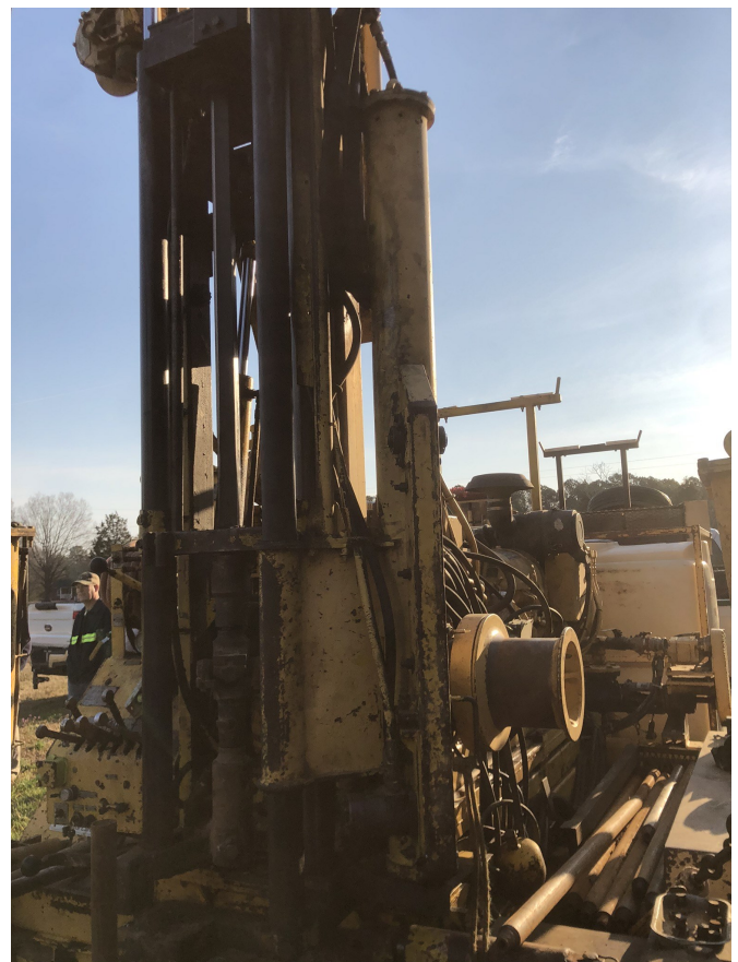
Figure No. 4: Automatic Hammer
