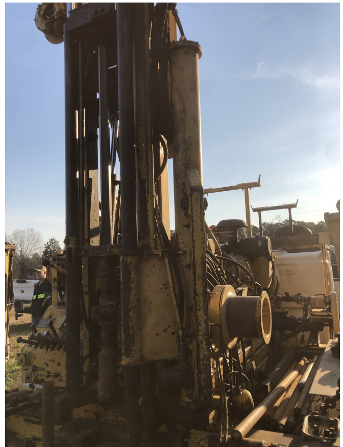
Figure No. 4: Automatic Hammer
