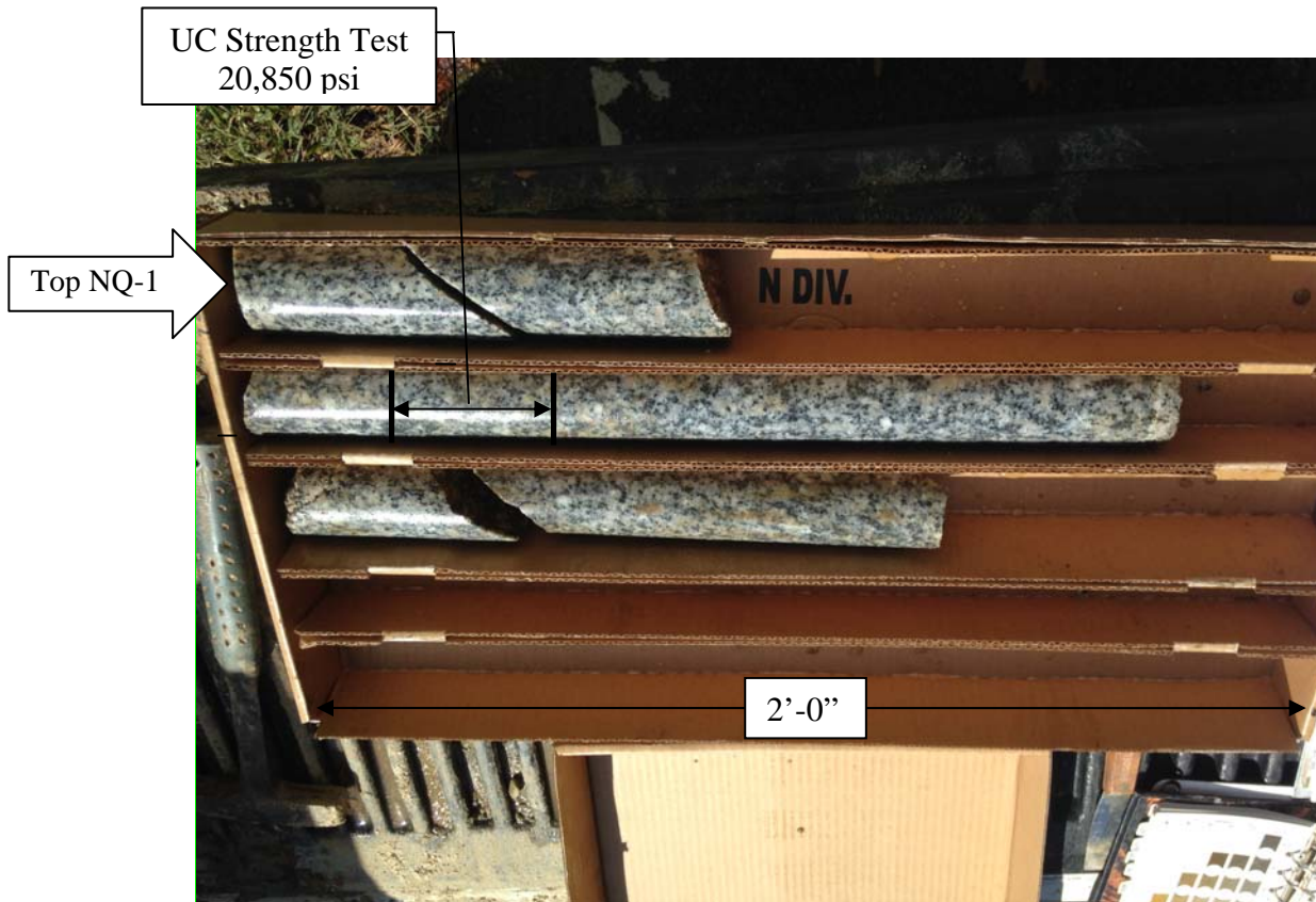
Photo 1. B-1 Rock Core Specimens NQ-1
