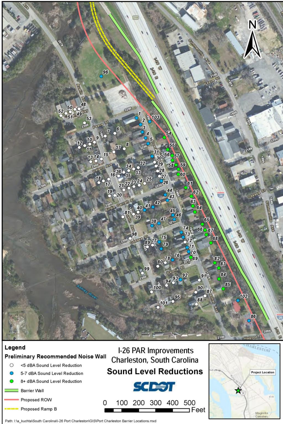
Figure 3 – Preferred Noise Barrier Placement and Results
