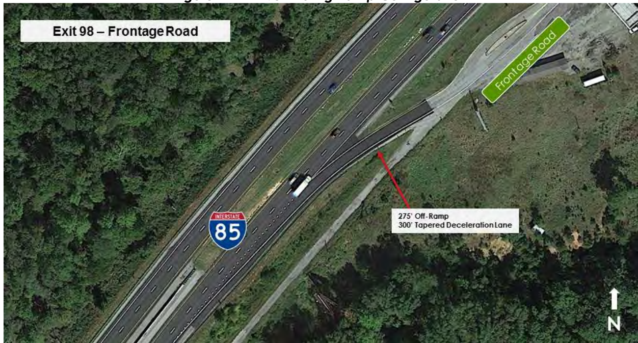
Figure 2 – Exit 98 Existing Ramp Configuration
