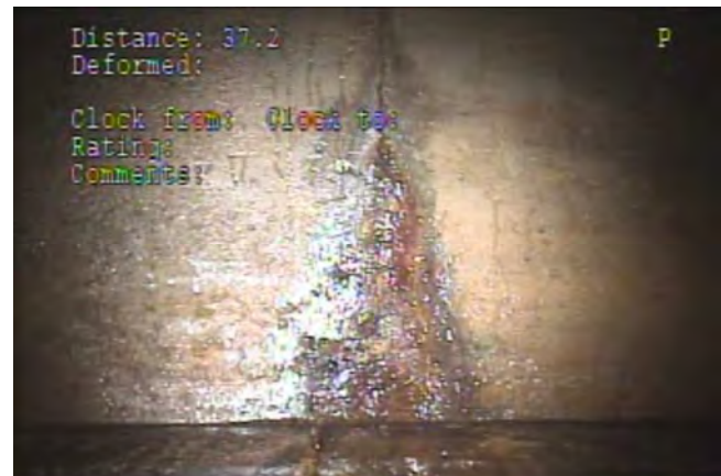
Joint issues/deformed at 37 ft
