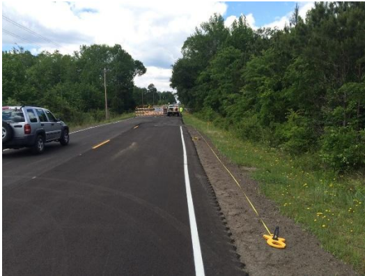
13. Photograph of MASW Array Back Swamp Bridge
