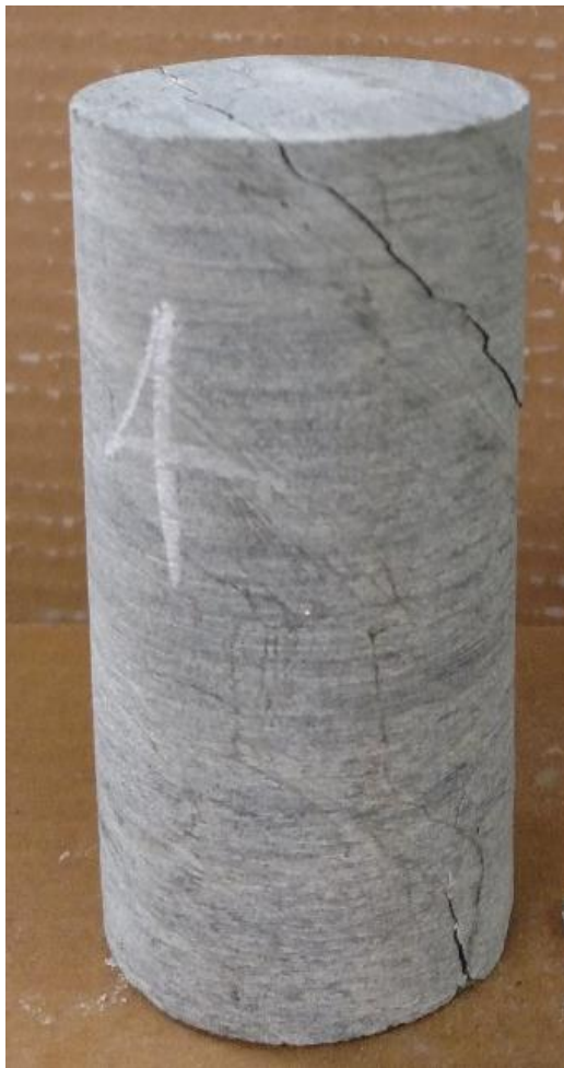
Core No. 4 UC Strength = 2,842 psi
