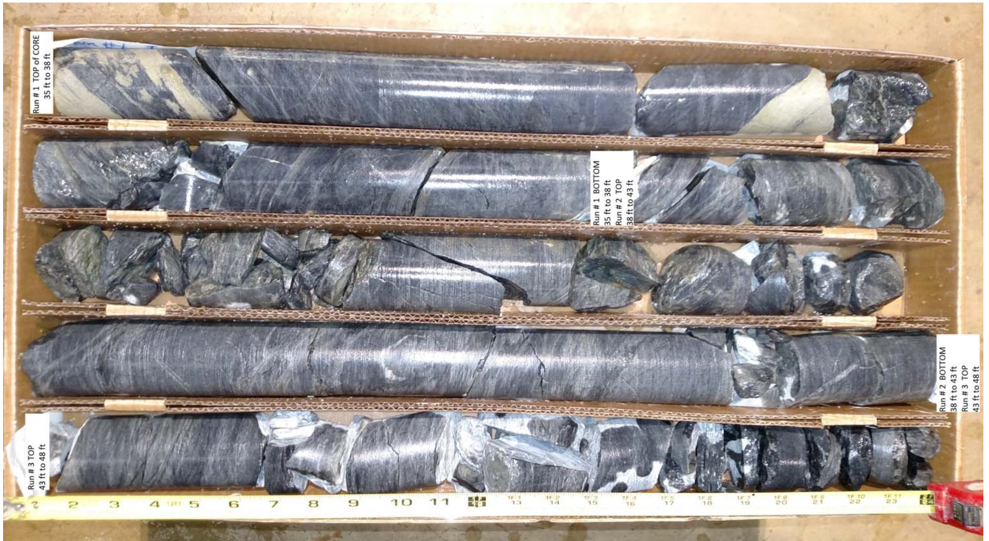
Figure No. 5A Rock Core Photographic Log S-28-36 Pine Grove Road, Kershaw County, South Carolina
