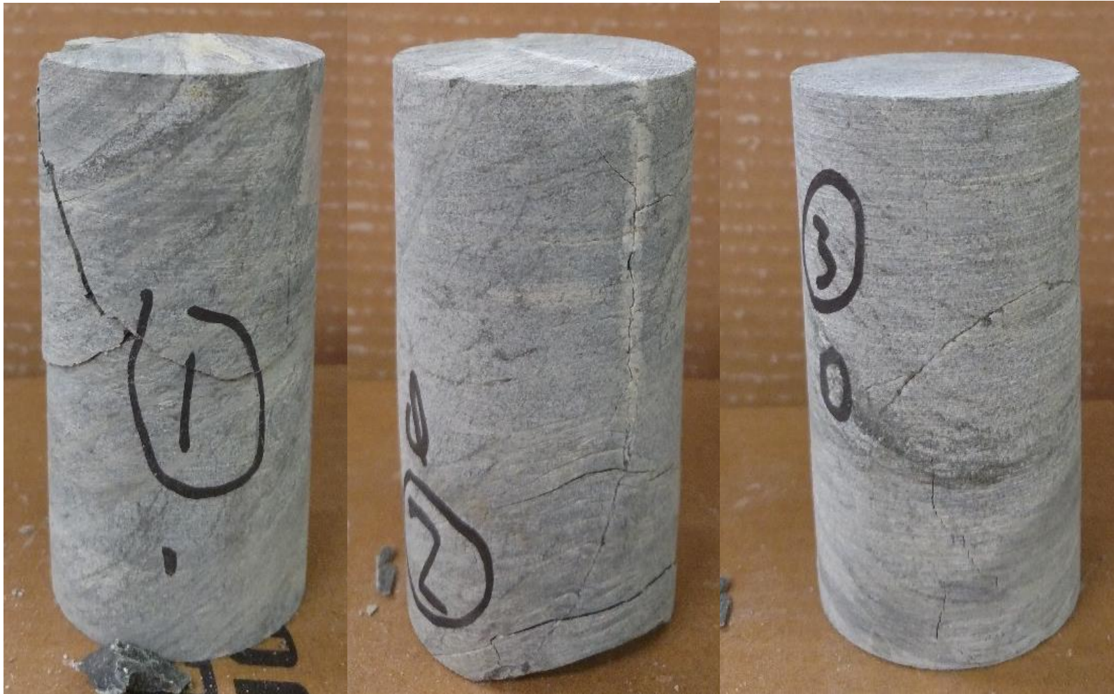
Core No. 3 UC Strength = 3,850 psi
