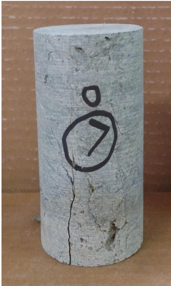
Core No. 7 UC Strength = 8,742 psi
