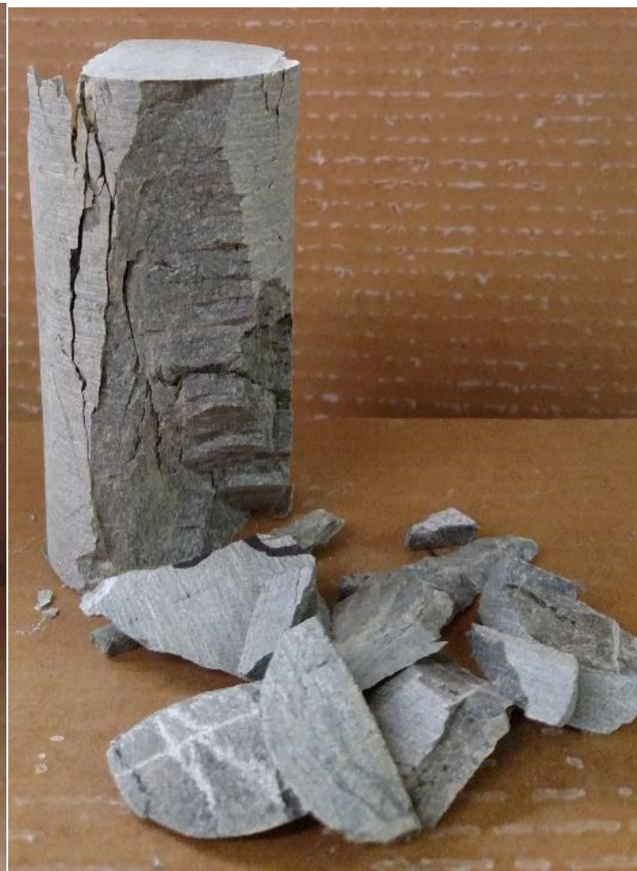
Core No. 8 UC Strength = 14,157 psi
