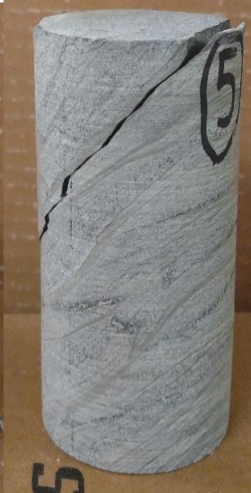
Core No. 5 UC Strength = 3,202 psi
