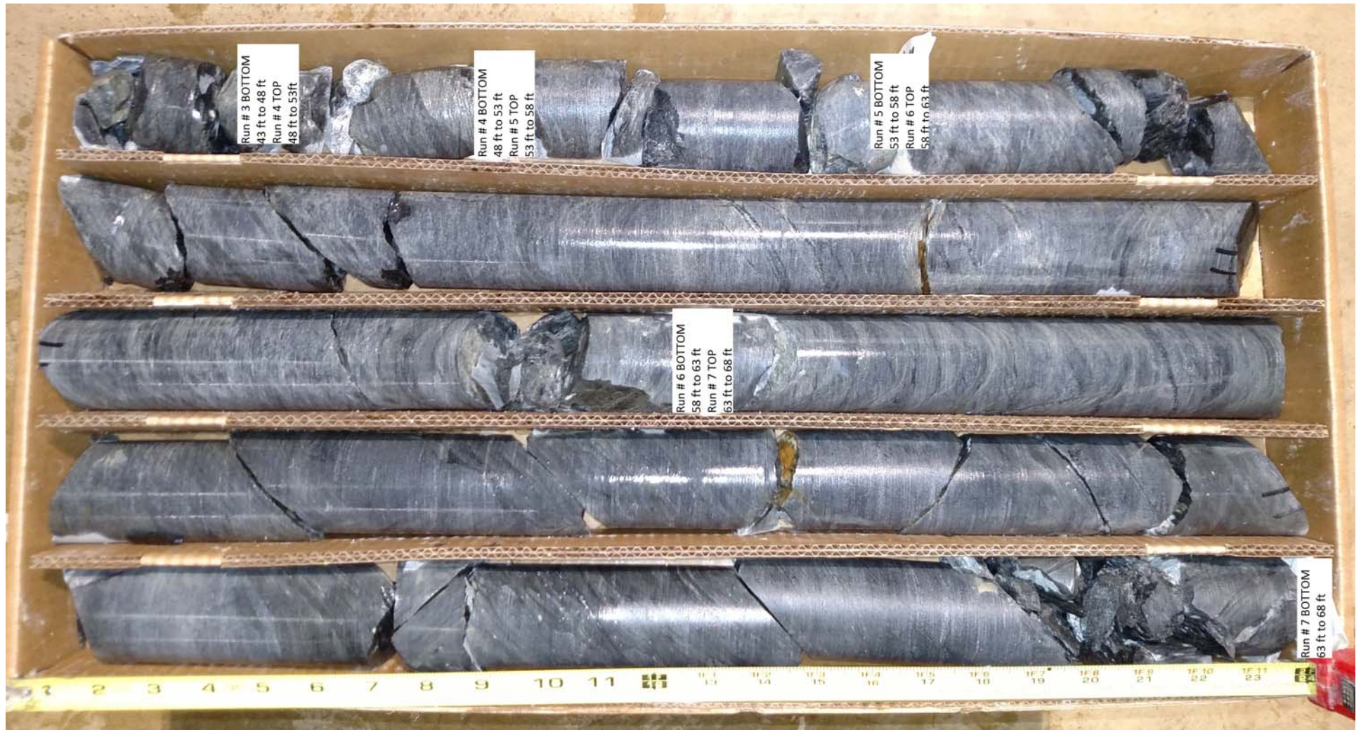
Figure No. 5B Rock Core Photographic Log S-28-36 Pine Grove Road, Kershaw County, South Carolina
