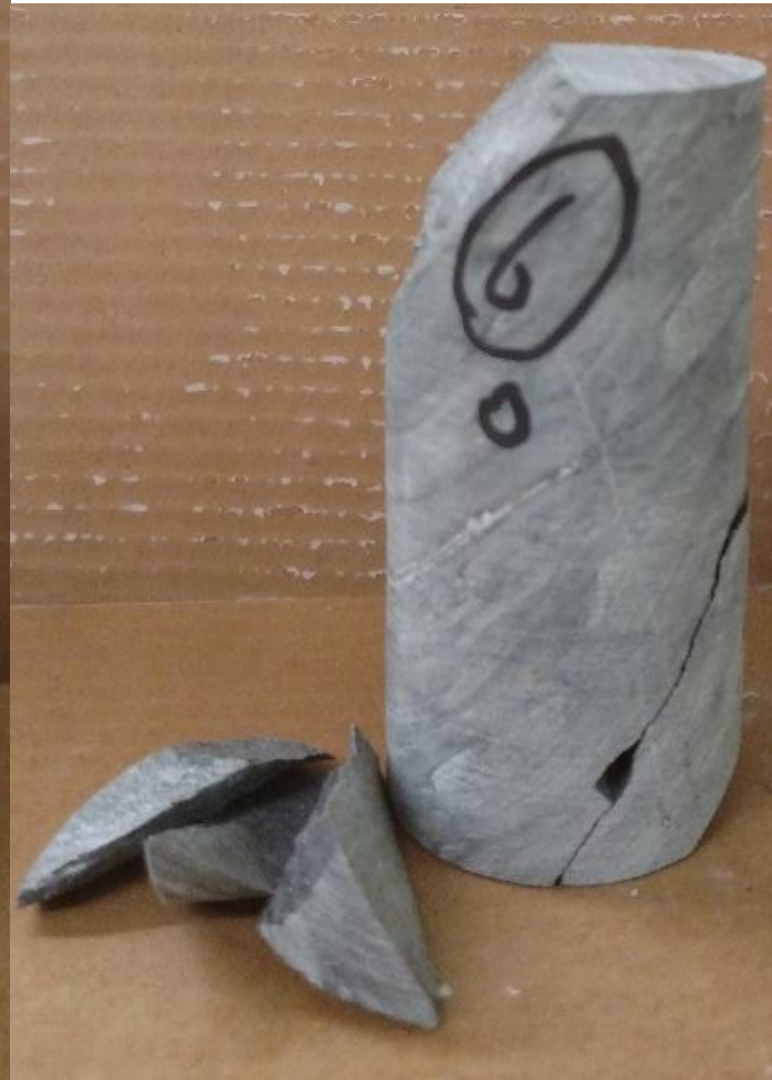
Core No. 6 UC Strength = 3,641 psi
