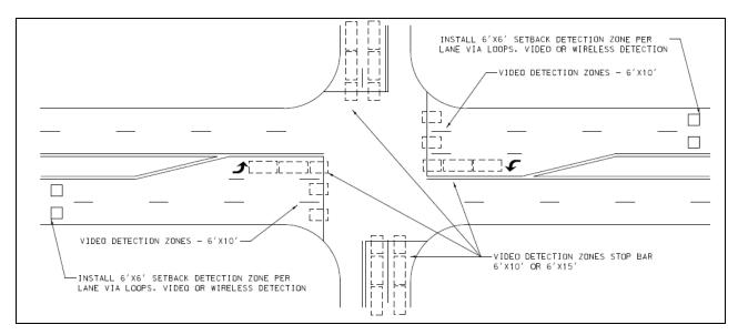
Figure 4-6 Video Detection Zones for Traffic Adaptive
