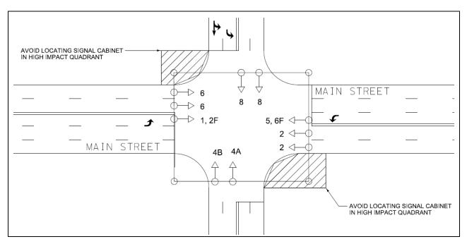
Figure 4-2 High Impact Signal Cabinet Locations
