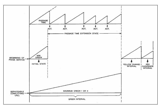
Figure 2-4 Typical Standard Timing Diagram
