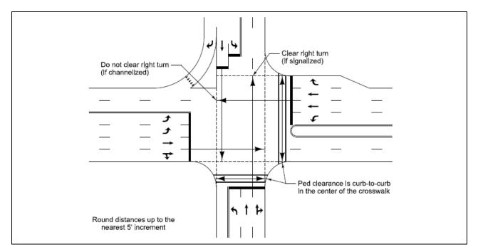
Figure 2-8 Through Movement Clearance Distances
