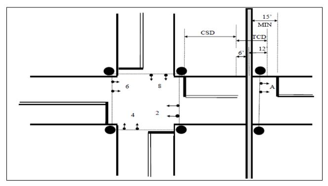
Figure 5-2 TCD and CSD Measurement Guide
