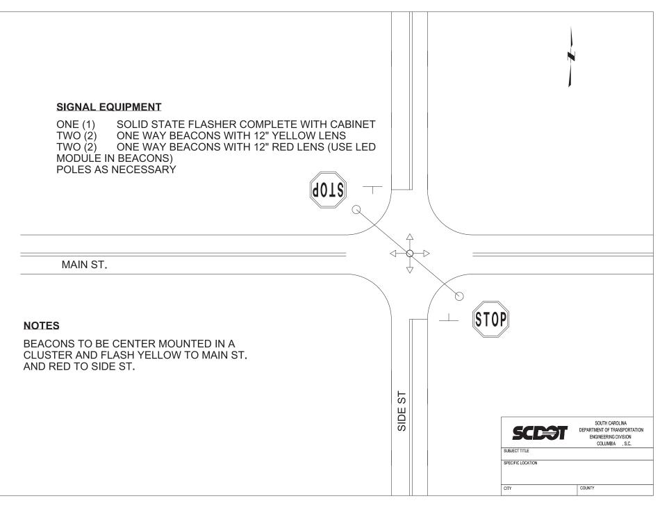
Figure 6-2 Cluster Overhead Intersection Beacon
