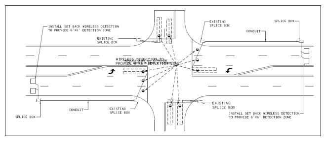
Figure 4-5 Wireless Detection with Inductive Loops for Traffic Adaptive
