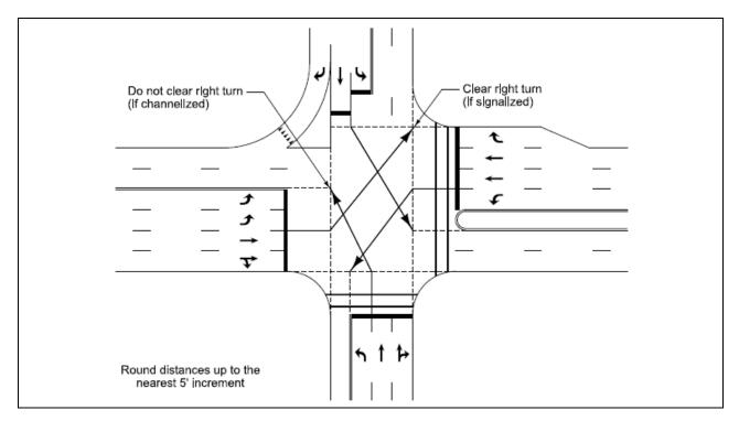
Figure 2-9 Left Turn Movement Clearance Distances
