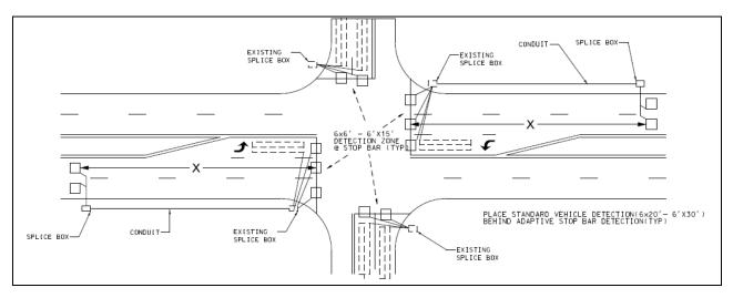
Figure 4-3 Inductive Loops for Traffic Adaptive
