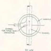
FORCE MAIN CONNECTION DETAIL
