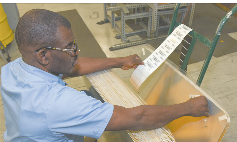
Donnie Mack adds barcodes to finished signs. The barcode helps SCDOT keep up with the inventory of approximately 750,000 highway signs across the state. In addition to recording the sign's location, the barcode also puts a date on the sign to schedule the signs 10-year life cycle.
